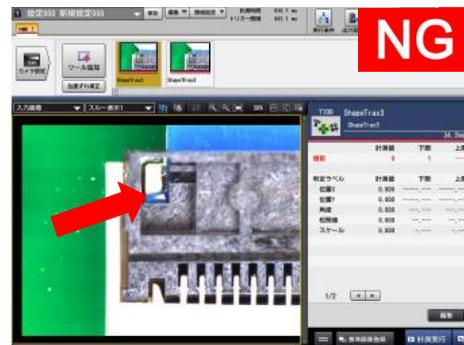
Test result by an image processing device maker
